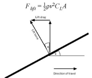
The horizontal component causing lift drag is thus:
