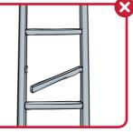
Never use a ladder with missing, broken or loose parts.
