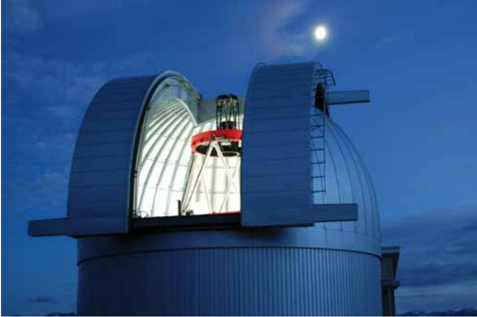
The MOA telescope at Mt John by moonlight. With a diameter of 1.8m it is New Zealand's largest telescope. [Courtesy Takashi Sako, Nagoya University.]
