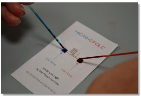
Example of a paper microfluidic "Tron race" that tests how far a liquid travels in a given period of time, for a particular shape of track.
