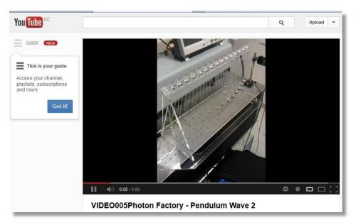
Pendulum wave demonstration built in response to student suggestion. Students time the wave oscillations. $^{5}$
