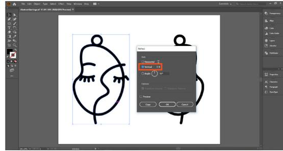
11. Prepare your design for laser cutting. For both earrings, change the stroke colour to red (RGB 255,0,0) and the stroke weight to 0.001.
