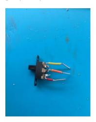
Figure 6: Jumper Wires soldered to the switch.
