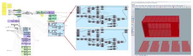
Figure 4. On Left the xUI Grasshopper description; Centre a detail of its complexity; On right a screenshot of the xUI building the model and its components
