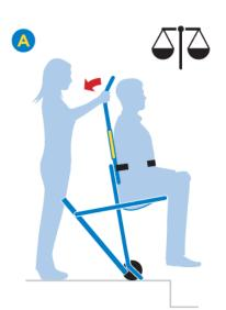
On reaching the summit of the stairs, rear wheel assembly can now be closed and frame of chair tilted into balance position.
