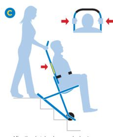
After the chair has been pushed onto the stairs ensure the tracks make contact with the top two stairs and pause. The friction tracks will hold the chair to the stairs.
