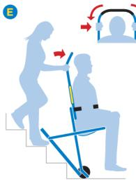
As the front wheels touch the floor at the end of the stairs, move hands back to side of handle and tilt chair forward.
