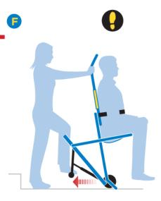
On reaching a level surface rear wheel assembly can now be released ready for horizontal travel.
