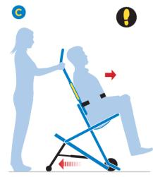
To easily transport the passenger to the top of the stairs, use your foot to deploy the rear wheel assembly.
