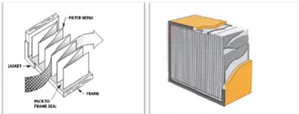
Figure 5: HEPA filter construction
