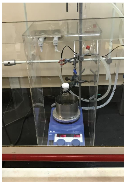
Figure 1: Ideal use and set up of a blast shield. Note that the combination of fully lowered fume hood sash and blast shield assist in containing any potential explosion.
