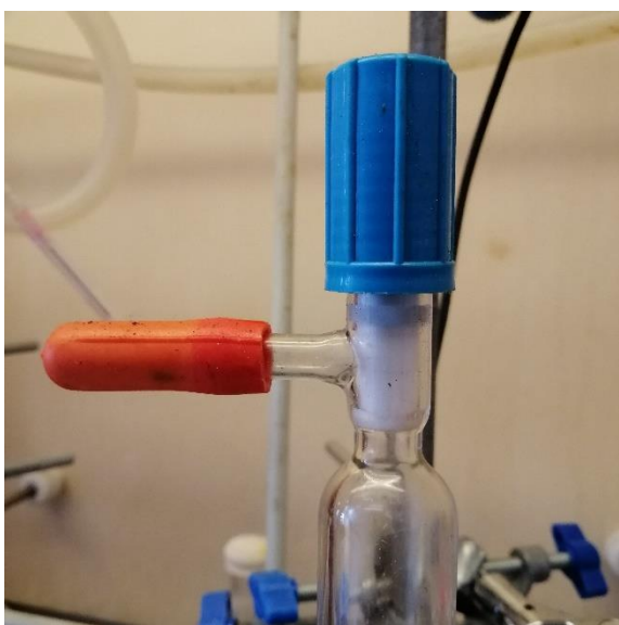
Figure 2: Example of a sealed reaction vessel that is NOT suitable for pressurised reactions.
