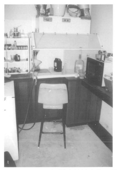
Fig. 1. Photograph of the fume cupboard where the spill of 70% w/w hydrofluoric acid occurred. Note the restricted space of the fume cupboard, the digestion cup and 2-l. bulk hydrofluoric acid container.
