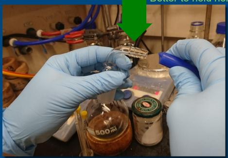
Pay extra attention and do not use excessive force when attaching rubber tubing to glass! This includes gas adaptors, manifolds or any other weak joints. Rotate the joining partners with steady pressure or use a tiny smear of grease (*if appropriate for your work*).
