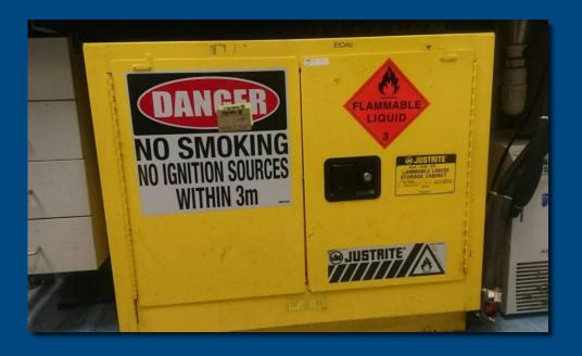
Make sure all solvents not in use are returned to the solvent cabinets, especially when leaving the lab.
