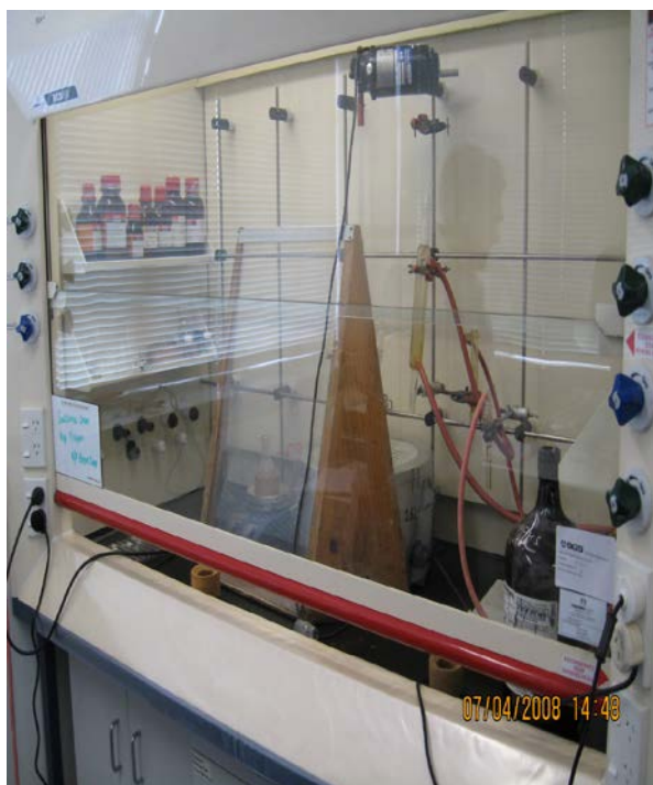
Figure 1: Ideal use and set up of a Blast Shield. Note that the combination of fully lowered fume hood sash and Blast Shield assist in containing any potential explosion.
