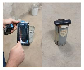
Once the canisters were fully packed, the external radiation levels were measured to ensure the safety of those dealing with the transit and disposal. The drums were then packaged, and we moved onto the next step of regulatory disposal via the Office of Radiation Safety. A third radium source at Faculty of Health and Medicine Sciences (FMHS) was also packaged for disposal at the radioactive bunker in FMHS.
