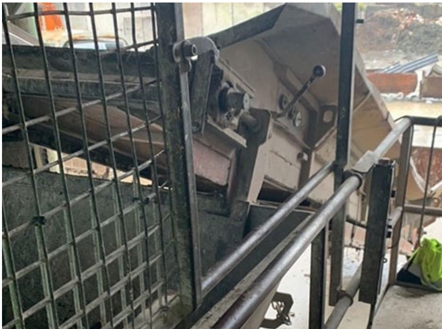
The unguarded waste shredder at M E Jukes and Son in Gisborne.
