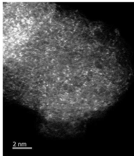
Scanning transmission electron microscopy image showing iron single atoms (bright spots) on an N-doped carbon support. The 2 nm scale bar corresponds to 1/40000 the width of a human hair.
