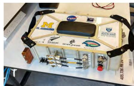
The Rongowai payload freshly arrived in Aotearoa, about to undergo bench testing at the University of Auckland.
