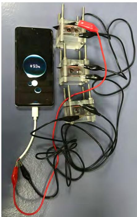
A smart phone being charged by three zinc-air batteries connected in series, each using an iron single atom catalyst (Fe-N-C) for ORR during battery discharge.
