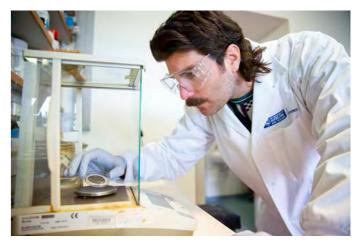
Dr Joel Rindelaub weighs out filters on the analytical balance to perform gravimetric analysis of aerosol mass loading. Photo: Elise Manahan
