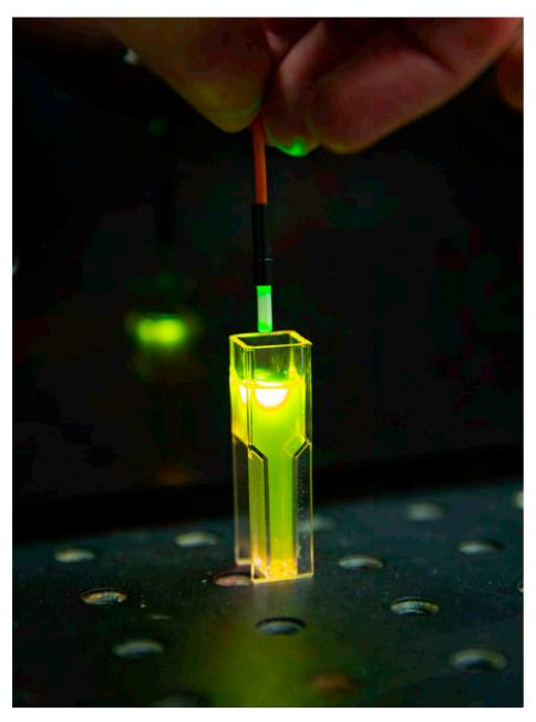
Fluorescence in action. Fluorescence is the process when a material absorbs light and emits light of lower energy. Here a rhodamine solution absorbs green light to emit yellow light. The phenomenon of fluorescence is used by the FoodSafe group to enumerate bacteria. Photo: Elise Manahan
