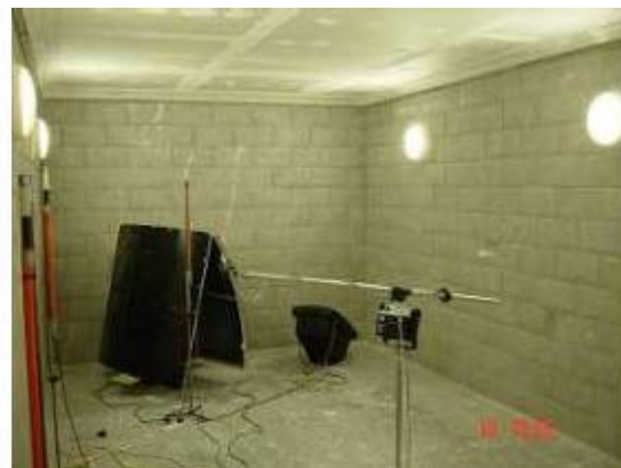
Figure 2 , Floor Test Rig, End dia. poles @ 600mm centres. Measuring the sound field
