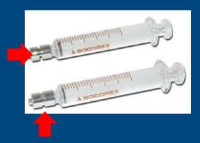
Luer lock syringes MUST be used for any transfer of toxic or corrosive reagents
