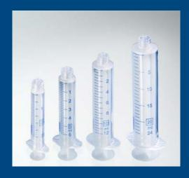
Syringes are used to safely transfer solvents and reagents into reaction vessels through rubber septa
