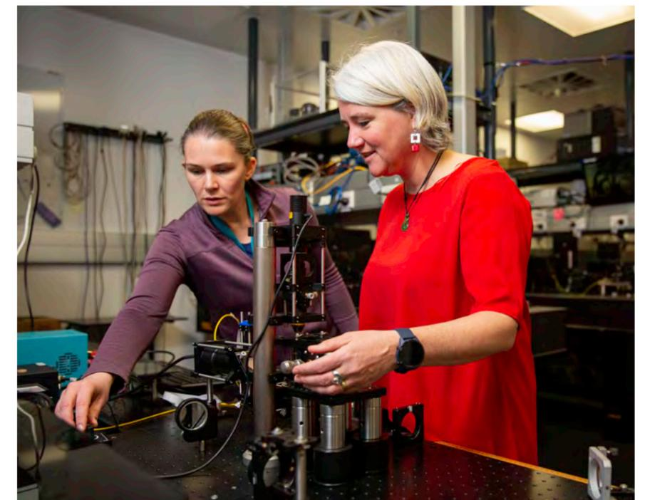
Associate Professor Frédérique Vanholsbeeck and Dr Cushla McGoverin assemble optical tweezers to allow for fluorescence studies of a single bacterial cell. Optical tweezers use light to hold in place and manipulate small particles such as a bacterial cell and therefore allow us to follow the same cell over time while changing the surrounding environment (e.g. media the cell is immersed in). Photo: Elise Manahan
