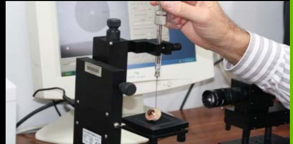
A water droplet is being syringed on to an artificial eye set up in a goniometer.
